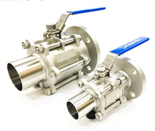
Anson offer PCW valves in full port for high flow and oil-free stainless steel for long service life. Our valves utilize 3-piece construction for easy maintenance, while a floating ball allows for positive shut-off. Wide range of sizes and end-connection options make it easier and lower cost for your cooling system.
